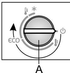
**Switching on:** To switch on: rotate the **A** dial clockwise.
