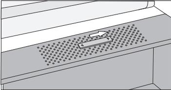
**Slider position to the right:** closed vents, higher humidity in the bin
