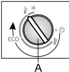
If the temperature of the room where the appliance is installed is below 16 °C, we recommend setting the **A**
