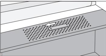
**Slider position to the left:** open vents, lower humidity in the bin
