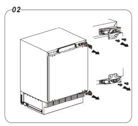
3. Turn the hinge over and place it on the diagonally opposite comer of the cabinet. Screw back in place. Repeat with the other hinge. Replace the door and re-attach the hinges. Check that the door is aligned horizontally and vertically and that the door seals are secure on all sides before finally tightening the hinge bracket screws.
