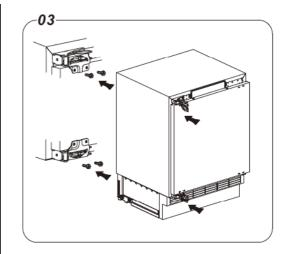
4. Replace the upper hinge cover (left and right). Replace the lower screw hole cover for the cabinet. Replace the screw hole cover for the door.
