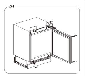
2. With the door closed, remove the screws on the outside of hinges. Open the hinges away from the door. With the hinge open undo the screws holding it to the cabinet. Be careful with the hinge, use a long shafted screwdriver if you have one.
